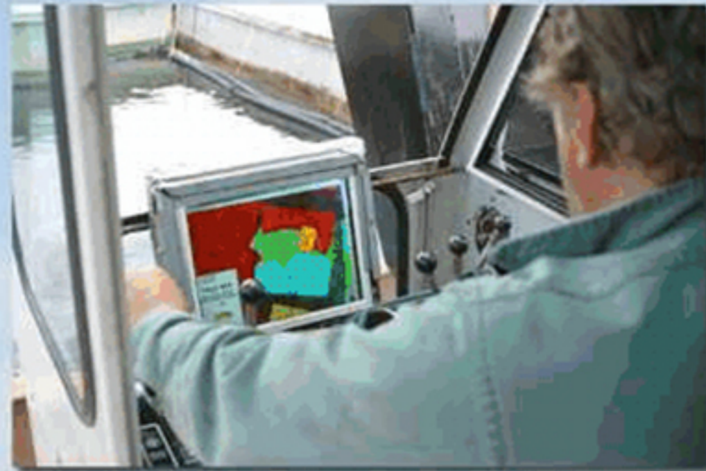
CLAMVISION positioning system guides operator and logs information about every bite taken
