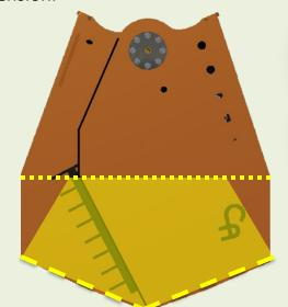
150° Cutting Edge allows the bucket to "scoop" material which lowers the materials center of mass within the containment area.
