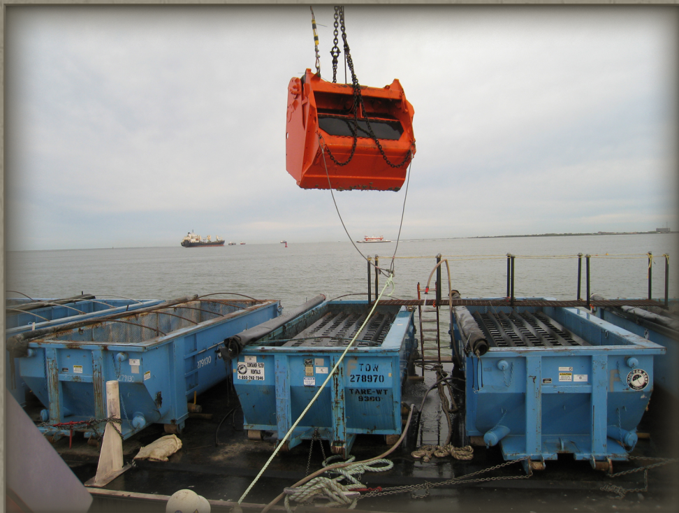
Image 4: Cable Arm Environmental Level-Cut Clamshell bucket
