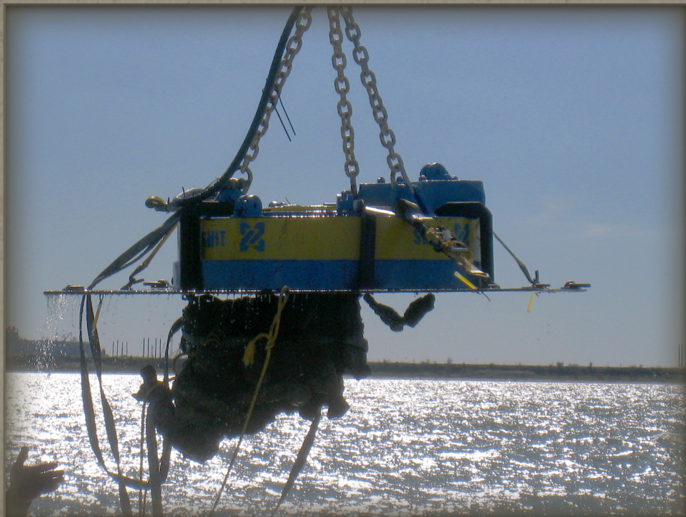
Image 3: Smit America's five feet diameter magnet
